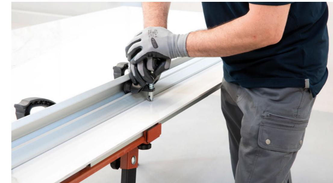
**NB:** Move the scoring carriage forward, applying constant pressure throughout the length of the cut.
