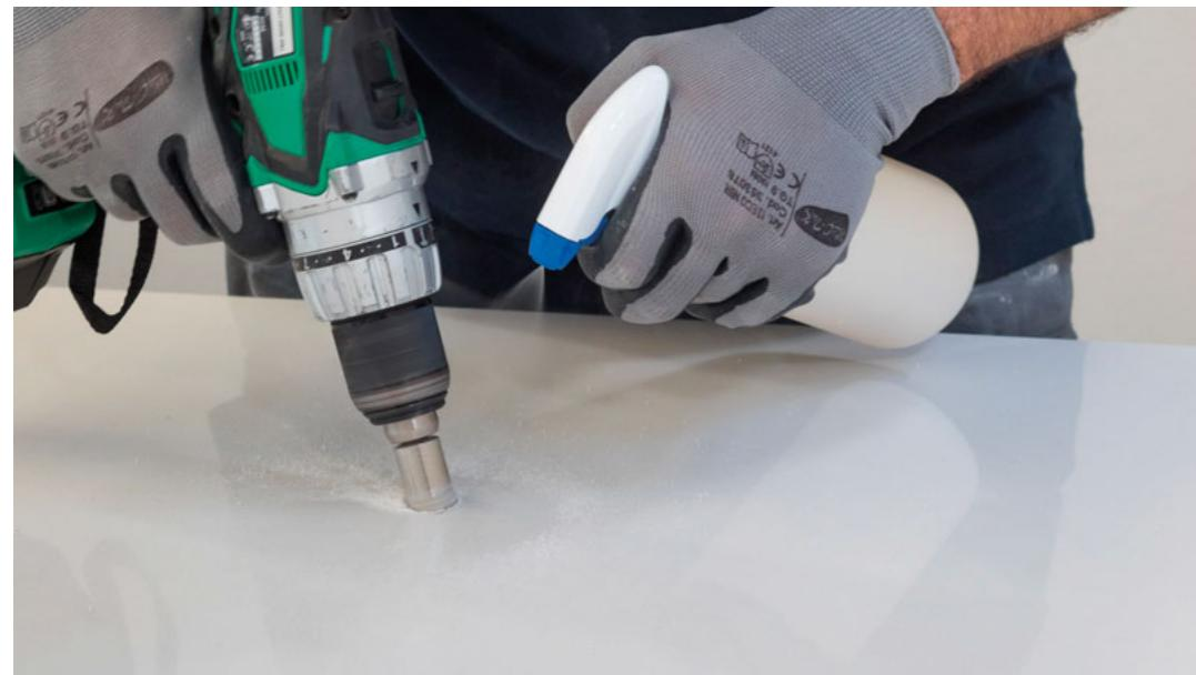
**2.** Drill the hole at an angle of 75°-85° to a depth of 1-2 mm into the slab.
