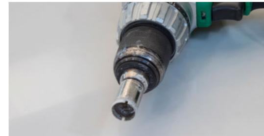
**Diamond core drilling bits** for wet drilling.
