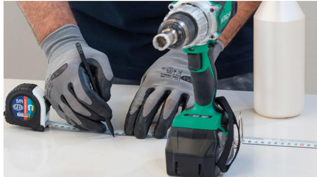
**1.** Place the Mega slab on a hard, firm, non-slippery surface such as wood or concrete. Wet the area where the hole is to be drilled with water.
