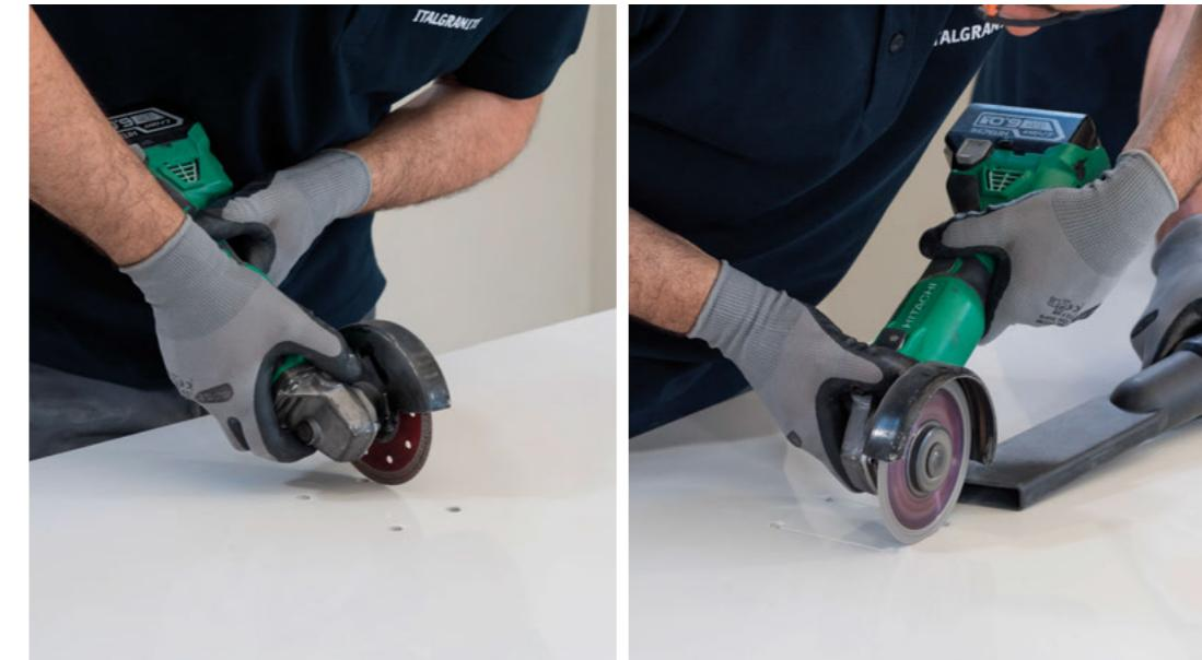
3. Cut the section between the hole and the end of the slab using an angle-grinder fitted with a diamond blade.
