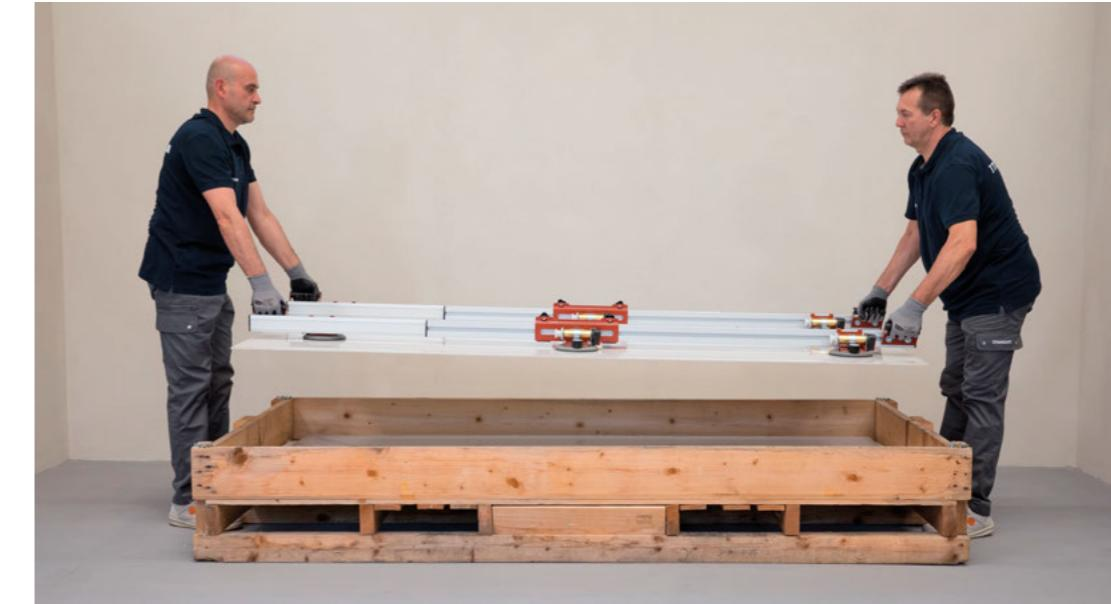
**3.** Lift the slab gently and place it on the workbench, or turn it to the vertical position and place it on the handling trolley for adhesive application.
