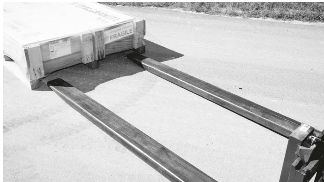
**B.** For correct handling of the pallet on the short side (e.g. when unloading containers), forks at least 2.5 metres long should be used to ensure that the material is held perfectly and safely.
